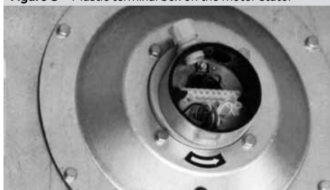
Figure 8 – Plastic terminal box on the motor stator
