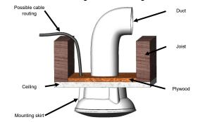
When surface mounting the iCON 30S, the mounting skirt provided should be used. The mounting skirt should be fixed, with the screws provided, into the support. The fan is then fitted into the skirt.
