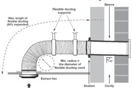
Where flexible ducting is used the diameter must be maintained and it is good ventilation practice that the ducting is extended to a minimum of 90% its possible length in order to maintain the best possible air flow.
