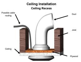
The fan should be fitted in the hole, fixed with the screws
