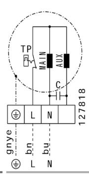
During operation, electric motors heat up. Under certain circumstances (excessively high ambient or fluid temperatures, heavy contamination, etc.), the motor temperature may exceed the safety limit of the electrically isolated parts. In order to avoid engine damage, various types of temperature monitoring are possible, of which at least one must be installed on site.
