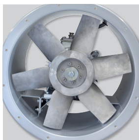
Impeller dynamically balanced Aluminium impeller manufactured from one piece casting. Dynamically balanced, according to ISO 14694: G6.3, giving vibration free operation.
