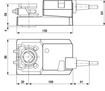
When using a round spindle made of CrNi (INOX): Ø 12...20 mm
