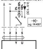
Control remotely 0...100% with positioner SG..
