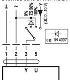
Control remotely 0...100% with positioner SG..
