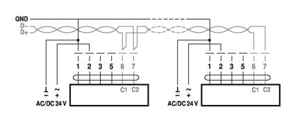
Cable colours: 1= black 2 = red 3 = white 5 = orange 6 = pink 7 = grey BACnet / Modbus signal assignment: C1 = D- = A C2 = D+ = B
