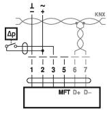
Requirements switching contact: The switching contact must be able to accurately switch a current of 16 mA@24 V.  depending on type
