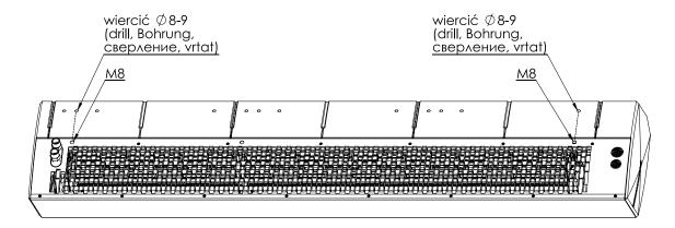
Drawing below shows the position of the mounting holes for the pins
