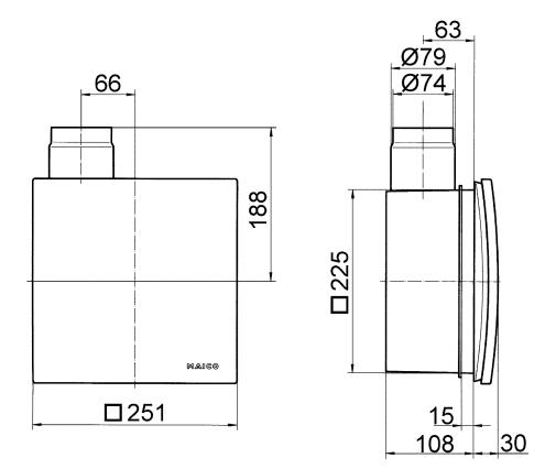
ER fan insert with recessed-mounted housing ER-UP/G or ER-UPD
