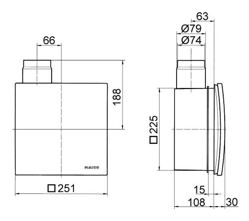
ER fan insert with recessed-mounted housing ER-UP/G or ER-UPD
