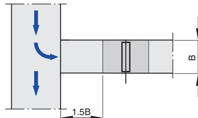
The stated volume flow rate accuracy  $\Delta q_v$  can only be achieved with a straight duct section of at least 1.5B upstream between any bend and the controller.
