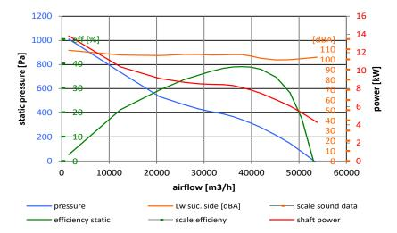
Measured in short casing with bellmouth without guard grille in installation type A according to ISO 5801.
